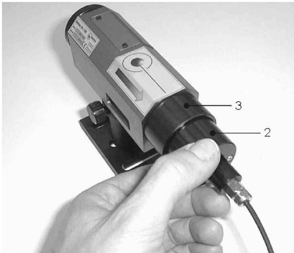
**Figure 6** Fine adjustment of mirror spacing
