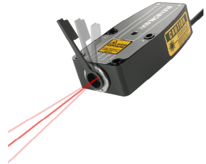
Renishaw's RLE10 laser encoder provides simple 'bolt down and dial in' installation thanks to fibre optic laser delivery and an integral beam steerer in the RLD detector head
