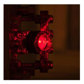
Note: The goal of this step is to ensure that the red beam can pass through the tube by being as far away as possible from any obstructions (as close to the bore axis as possible), and the entry point on the HR mirror should be chosen to satisfy this condition. The most likely objects to cause obstructions are the bore ceramic and the filament, and this can be probed. To assess how far the beam is from these obstructions, the adjustments of the He-Ne platform should be used.
