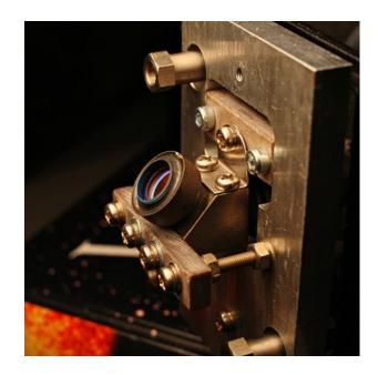
The prism seems to be a double-pass with an HR mirror set at an approx. 45 degree angle. The optical axis is offset from the center of the HR mirror, on the following photograph an image of the filament and the bore can be seen, refracted by the prism:
