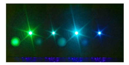
Anode current was set to approx. 5.5A. The exposure in each frame was the same, so the intensity is comparable. The 488nm line was stronger than the 514.5nm, most likely because this laser model was optimized for 488nm.
