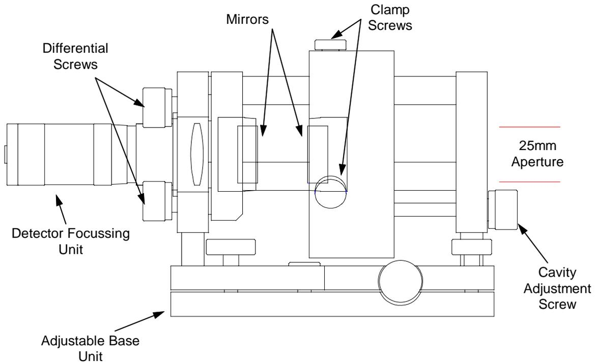
This, the most important component, houses the optics and the piezo-electric transducers which scan them. It consists of an Invar tri-bar structure supported by two Invar end plates.
