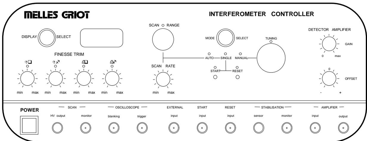
This component, generates and supplies the high voltages necessary to govern the movement of the mirrors in the optical head. DC components for mirror parallelism and tuning of the etalon are supplied when the head is in the MANUAL mode, and a ramping component is superimposed on these when in the AUTO or SINGLE mode. Provision is also made for the application of an external control signal, which would then be superimposed on any internally generated voltage.
