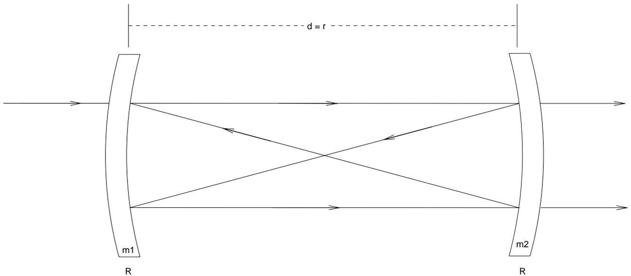
The confocal Fabry-Perot as illustrated above is formed by two spherical mirrors separated by their radius of curvature. The analysis of the operation is broadly the same as that for the planar etalon. There are some significant differences however :
