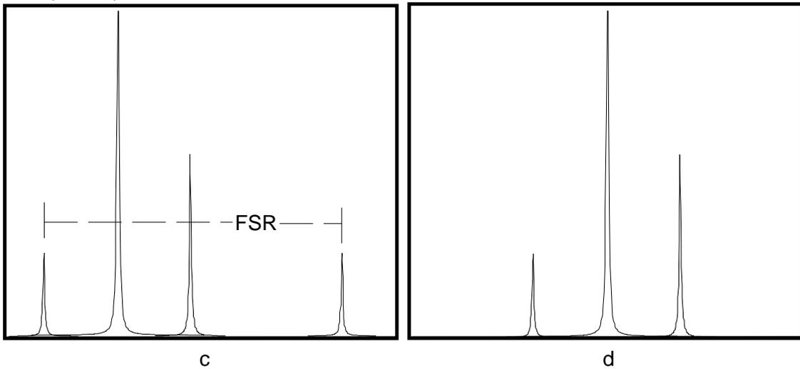
From trace d we can see that in this example the spectrum consists of three evenly spaced modes of different intensities, which is typical of the output of, for example a HeNe laser. The mode separation, and the relative amount of power in each mode can thus be assessed, and with the aid of a polariser their planes of polarisation can be deduced.
