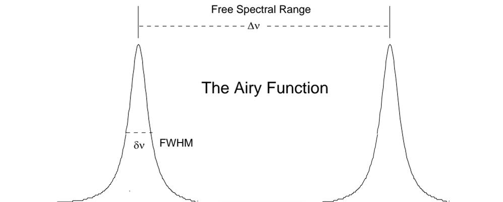
The airy function is obviously cyclic, due to the  $\sin^2$  term. The period of the function, known as the *free spectral range* is given by:
