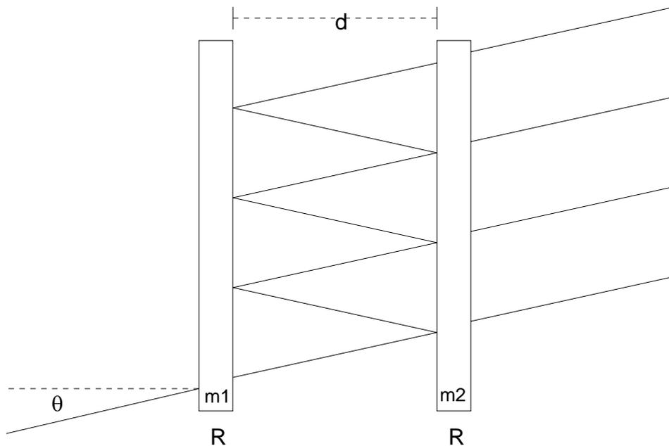
The planar system, as illustrated above, consists of two flat mirrors of reflectivity R. Light enters from the left at an angle  $\theta$ . The multiply reflected beams interfere, with constructive interference, and thus resonance occurring when the beams are all in phase with one another at the second mirror m2.
