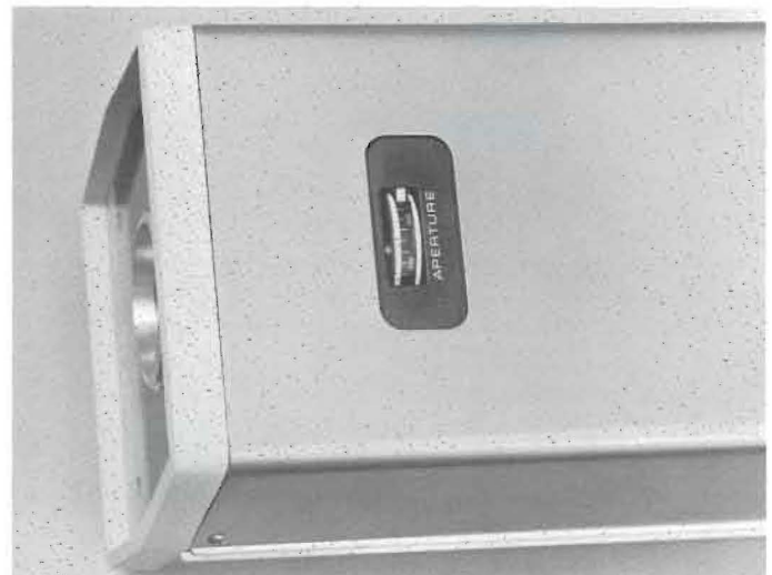
Figure 4 Intra-Cavity Aperture Control for Power and Single Mode Selection
