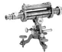
Fig. 2: Levelling Instrument from 1870
