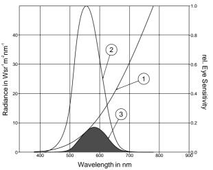
Fig.19: Determination of  $K_m$ , (1) calculated due to Planck's formula at  $T{=}2045^0K,$  (2) sensitivity curve of the human eye, (3) product of both curves
