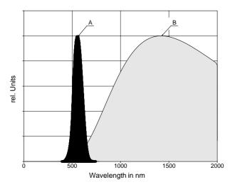
Fig.18: Sensitivity curve of the human eye for day view (curve A) and Planck's energy distribution of a black Platinum radiator at its point of solidification of 2048 K (curve B)
