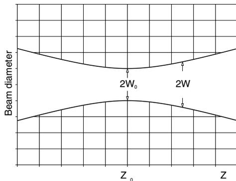
**Fig. 4.2: Beam diameter of a Gaussian beam as fundamental mode TEM<sub>00</sub> and function of z.**
