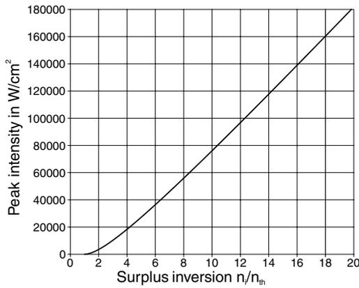
**Fig. 1.11: Attainable peak intensity of the cw Nd YAG-Laser at T=1% in Q-switch mode**
