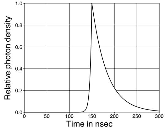
**Fig. 1.9 :** Calculated photon density for  $n_i / n_{th} = 10$ , a resonator length  $L$  of 100 mm and resonator losses of 1%. The rising part of the curve corresponds to the surplus inversion and the falling one to the photon life time inside the resonator
