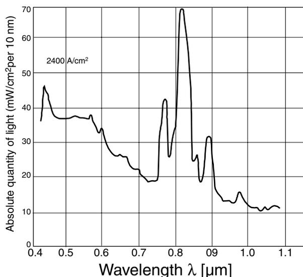
**Fig. 3.2 Emission spectra of a Xenon discharge lamp**
