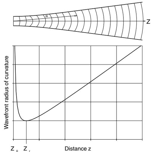
**Fig. 4.3: Course of the radius of curvature of the wave front as a function of the distance from the waist at z=0**
