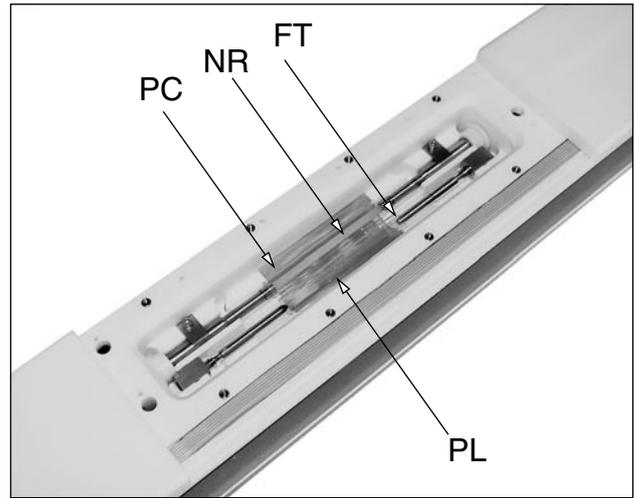
**Fig. 3.7: Pump cavity of the Nd:YAG Laser used**
