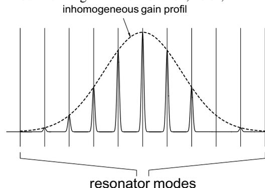
**Fig. 2.4: Inhomogeneous gain profile with shown resonator modes. Each individual mode has almost independent operating conditions within the group**
