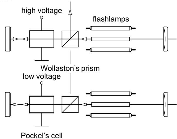
**Fig. 1.13: Electro-optical Q-switch device**
