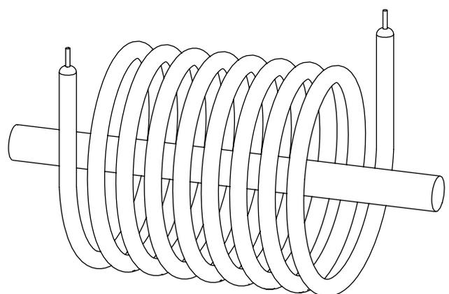
**Fig. 3.4: Helical ash lamp with Laser rod**
