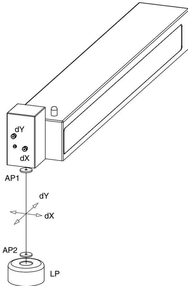
**Fig. A7.1: Checking Laser power**
