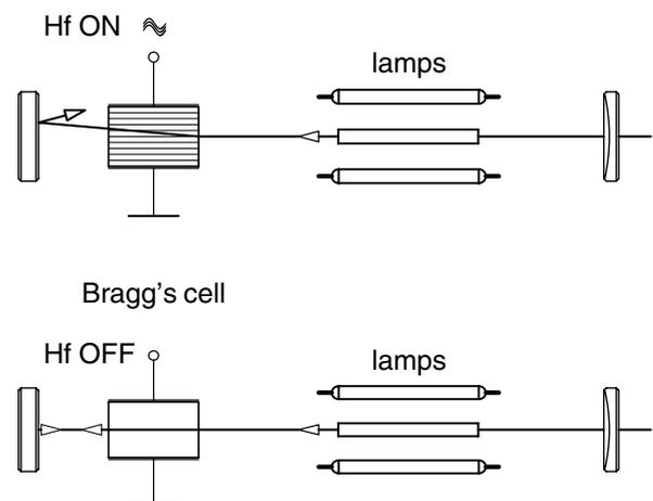
**Fig. 1.14: Acousto optical Q-switch device**
