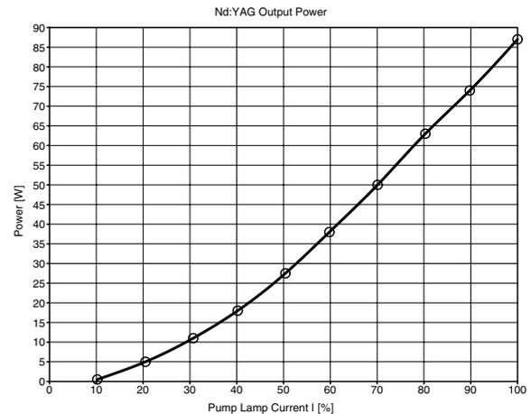
**Fig. A7.2: Laser output power versus pump lamp current**
