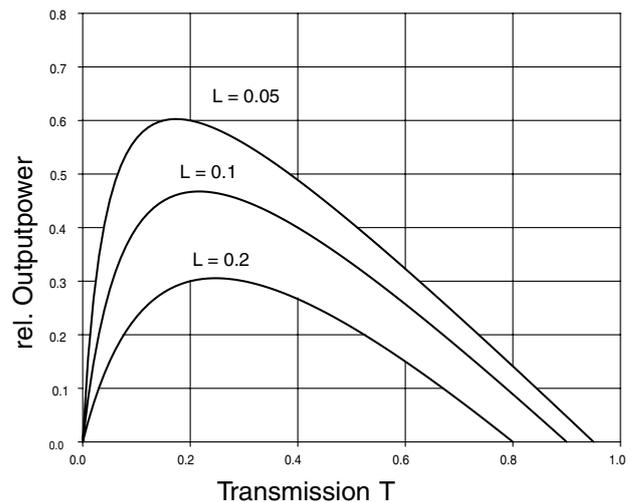
Fig. 1.7: Laser output power in dependence of the transmission T of the output mirror and the losses L.
