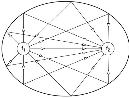
**Fig. 3.5: Ray tracing inside an elliptical cavity**
