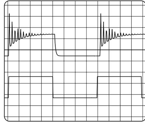
**Fig. 1.8: Spiking of the Nd-YAG laser**
