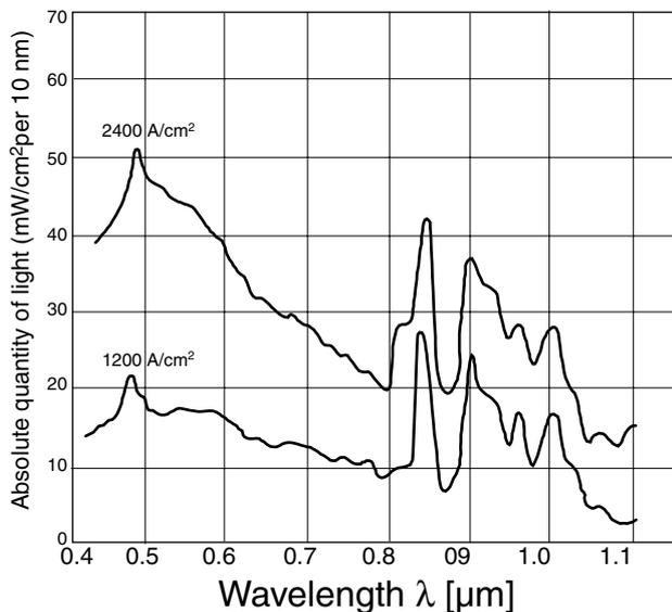
**Fig. 3.1: Emission spectrum of Krypton discharge lamps**
