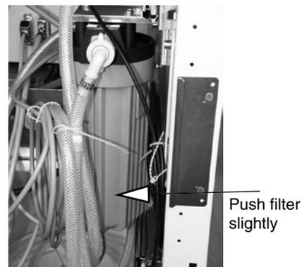
**Fig. A3.2 Pushing the de-ionisation filter**
