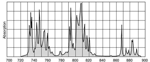
**Fig. 3.3: Absorption spectrum of Nd:YAG**
