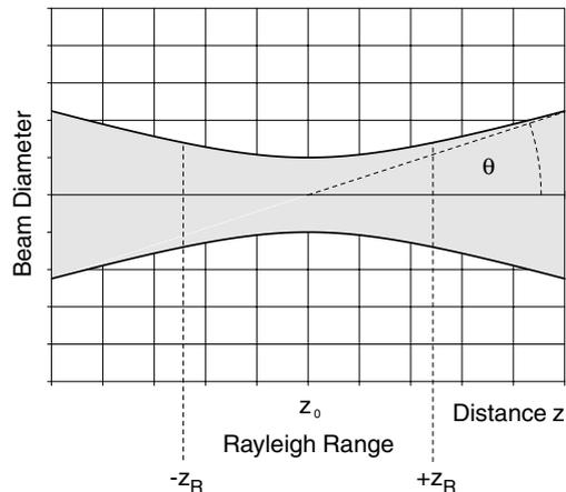
**Fig. 4.5: Rayleigh range Z<sub>R</sub> and divergence θ for the far field z >> z<sub>R</sub>**
