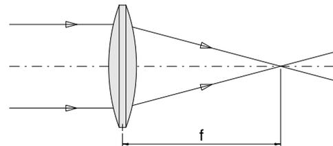
**Fig. 4.1: Focusing a beam in geometrical optics**
