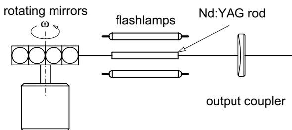
**Fig. 1.12: Mechanical Q-switch with rotating mirrors.**
