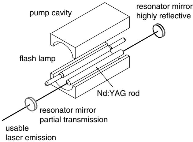
**Fig. 3.6: Arrangement of linear pump lamp and Laser rod**
