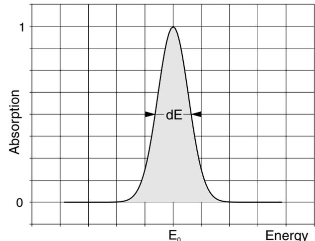
Fig. 1.2: Broadened absorption transition.
