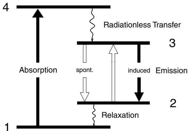
Fig. 1.5: Principle of the four-level laser
