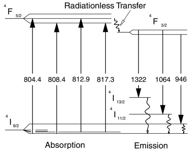
**Fig. 1.4: Relevant energy levels of Nd-YAG for optical pumping around 805 nm**
