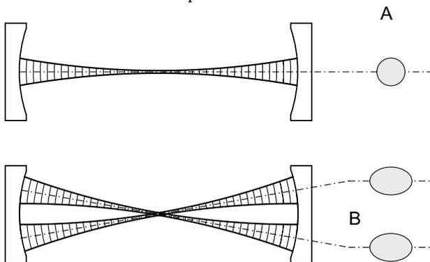
**Fig. 2.6: A spherical resonator with oscillation in the fundamental TEM<sub>00q</sub> (A) and a transverse mode TEM<sub>01q</sub> (B)**
