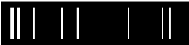
Fig. 13: Recording the emission of a light source with corresponding energy levels results in a line spectrum
