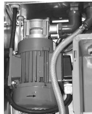
Fig. A4.1: Cooling pump marked with the right sense of rotation
