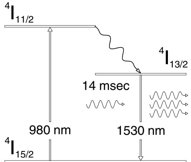
**Fig. 10: Three level system of EDFA**
