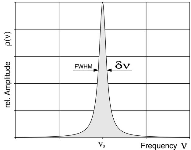
Fig. 5: The Fourier transformation of a damped oscillation as observed for spontaneous emission. It consists of the transition frequency  $\nu_0$  and a complete spectrum described by a Lorentz function.
